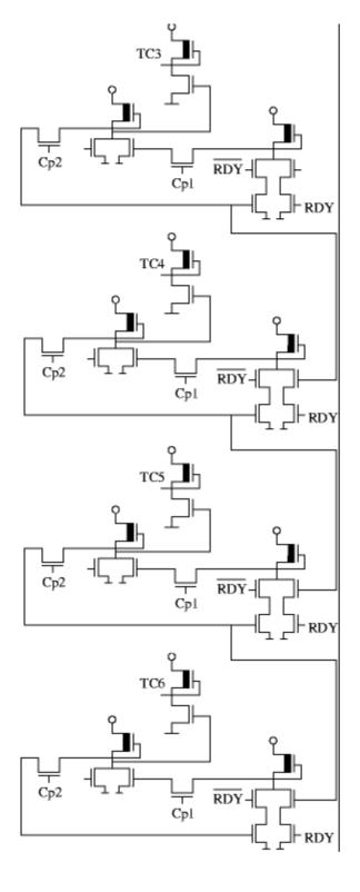
Its main task is to inform the instruction decoder about the clock cycle in which the instruction is during the executions need at least 2, max. 7 hours to terminate, the first cycle of which is always a fetch (that is, the loading operation code to the instruction register).
