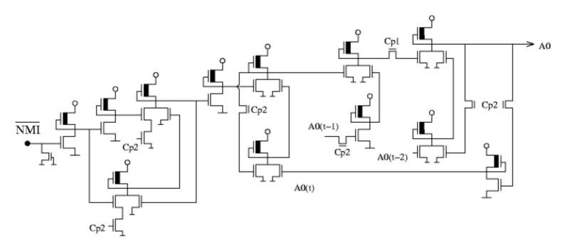
Seemingly it is only the Schmitt trigger input of the NMI that is directly connected to the above mentioned schematic works the same way in case of IRQ and RESET, since the lowest address pin is zero in all three cases, and the sig delayed by clock-cycle 1 and 2 drive this schematic
